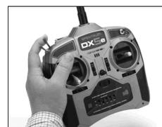
4. Follow the procedures of your specific transmitter to enter Bind Mode, the system will connect within a few seconds. Once connected, the LED on the receiver will go solid indicating the system is connected.
