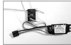
**Note:** To bind an aircraft with an electronic speed controller that powers the receiver through the throttle channel (ESC/BEC), insert the bind plug into the BATT/BIND port in the receiver and the throttle lead into the throttle (THRO) port. Proceed to Step #2.
